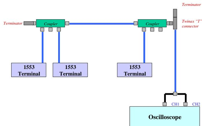
To connect to a STUB, there are several options. The simplest method is to connect your oscilloscope cable to an unused stub connection on one of your transformer couplers.
