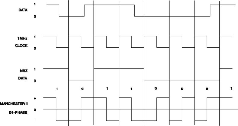
A transition signal occurs at the center of the bit time. A logic “0” is a signal that transitions from a negative level to a positive level. A logic “1” is a signal that transitions from a positive level to a negative level.
