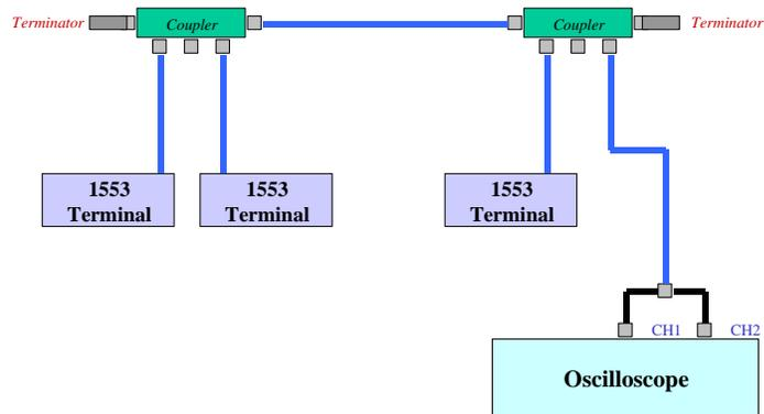
Another STUB connection method is to use a "T" connector to attach to a stub connection. To do this disconnect the stub cable from either the 1553 terminal or the bus coupler, connect the "T" connector in it's place, connect the stub cable to one end of the "T" connector, and connect your oscilloscope cable to the other end of the "T" connector.
