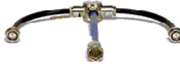
Once you have your adapter from the oscilloscope to the twin-axial cable, you need to connect it to your 1553 network. There are several ways you can do this, but in general you connect to the BUS or to a STUB. The examples below show connections to a transformer-coupled bus, but you can make the same type of connections if you are using a direct-coupled bus.
