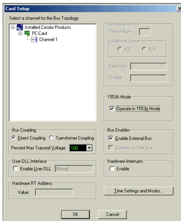
Select the option for **Operate in 1553A Mode**. This disables RT31 broadcast, disables SA31 mode code, and enables the decoder to see all commands.
