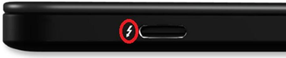
If the port is not labeled with the logo circled above, the port does not support Thunderbolt 3 and the adapter will not operate.
