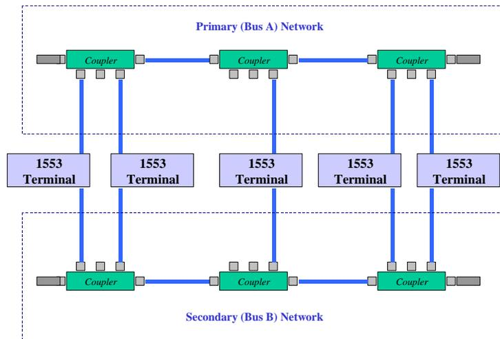
As you add terminals to your network, you can easily expand on the basic topology. Just remember to keep your stub lengths under 20 feet (or under one foot for direct-coupled stubs), and try to keep your bus length under 100 feet (don't use a 300 foot cable where a 20 or 50 foot cable will do). If you must use a longer bus, be prepared to deal with transmission line issues and propagation delay.
