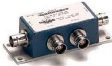
The bus coupler shown here is a *two-stub* coupler. It has two stub connections (on the side). The bus connections are on the ends. Bus couplers are available with one to eight (or more) stub connections. Be careful not to confuse bus connections with stub connections – a common mistake is to connect stubs to the bus connections or vice-versa.
