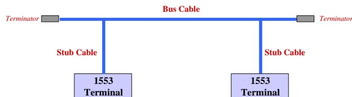
MIL-STD-1553 does not specify a maximum bus length, but as a general rule, try to keep your bus length under 100 feet. You can go longer but may have to deal with issues associated with propagation delay and transmission line effects.
