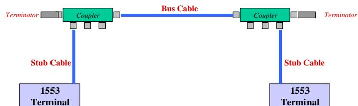
This is the *bare-minimum* 1553 network connection. A common mistake seen with basic connections between two devices is that someone tries to connect a cable from one device to another (with no terminators or couplers).
