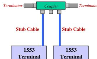
In the configuration shown above, the entire *bus* is inside the bus coupler. This is equivalent to using two separate couplers as shown in the following illustration:
