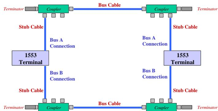
Be careful to keep the two networks separate – another common mistake is to inadvertently connect bus A and bus B together.
