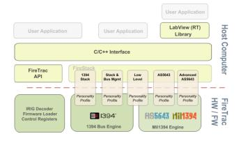
The Personality Profiles allow the solution to be adapted for use in embedded systems which typically have limited resources, and/or with powerful host processors that can utilize even the fully featured profile.
