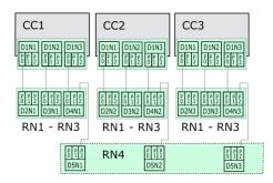
Other variants of how a single 3-node **FireTrac**<sup>®</sup> card can be used are depicted below. The left shows a CC devices simulating the triple bus interface (3 CC) whereas the right pictures demonstrates a possible single-branch usages model (CC + 2 RNs).
