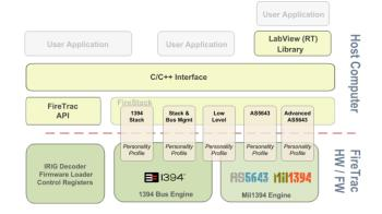
The Personality Profiles allow the solution to be adapted for use in embedded systems which typically have limited resources, and/or with powerful host processors that can utilize even the fully featured profile.
