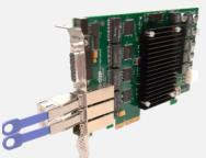
When enlarging the network, two or more FireTracs can be easily interconnected with SFF-SFF harnesses. Such harnesses are available in various lengths.
